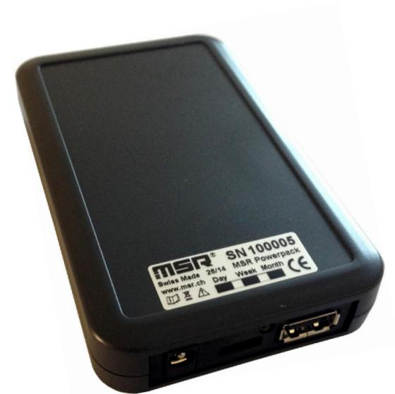
The MSR Power Pack is an autonomous charging station that can be used to recharge the internal battery of the MSR data logger during operation. Thanks to a capacity of 5000 mAh and an adjustable charging interval of one day, one week or one month, the unit is able to realise much longer measuring tasks. For instance, an MSR165 data logger is capable of realising measuring tasks that are up to 6 times longer.
