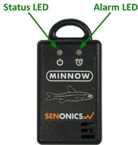
Figure 2: Minnow Alarm Indicators
