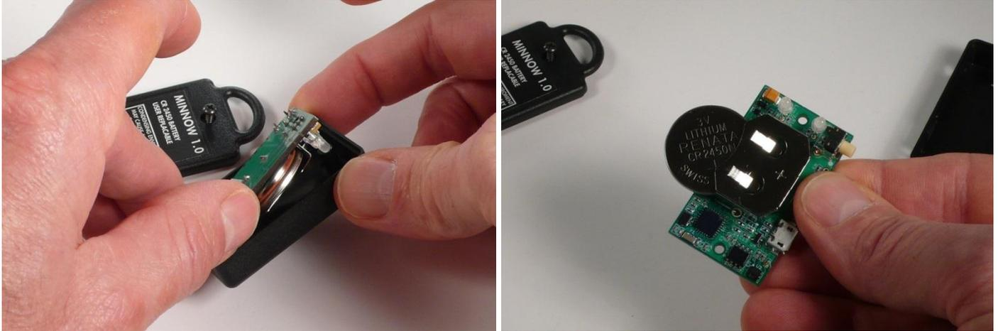
Insert a new battery as shown being careful not to touch and exposed electronics in the process. Finally re-attach the cover and tighten the fastener screws again (be careful not to over tighten).
