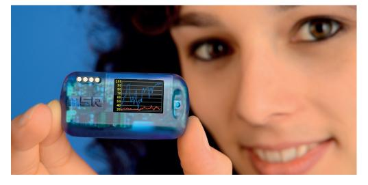
Wireless monitoring of measured data and fast readings of measured values – the new features of the Bluetooth Low Energy Option and the OLED graphic display of the MSR145 mini data logger. Also new: the web-based "MSR SmartCloud" service for mobile data monitoring.
