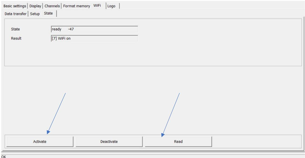
If the "ready" and "WiFi on" indicators for status and result appear, the logger is successfully connected to your WiFi connection and the local server (background process of the application) and the measurement data is sent.
