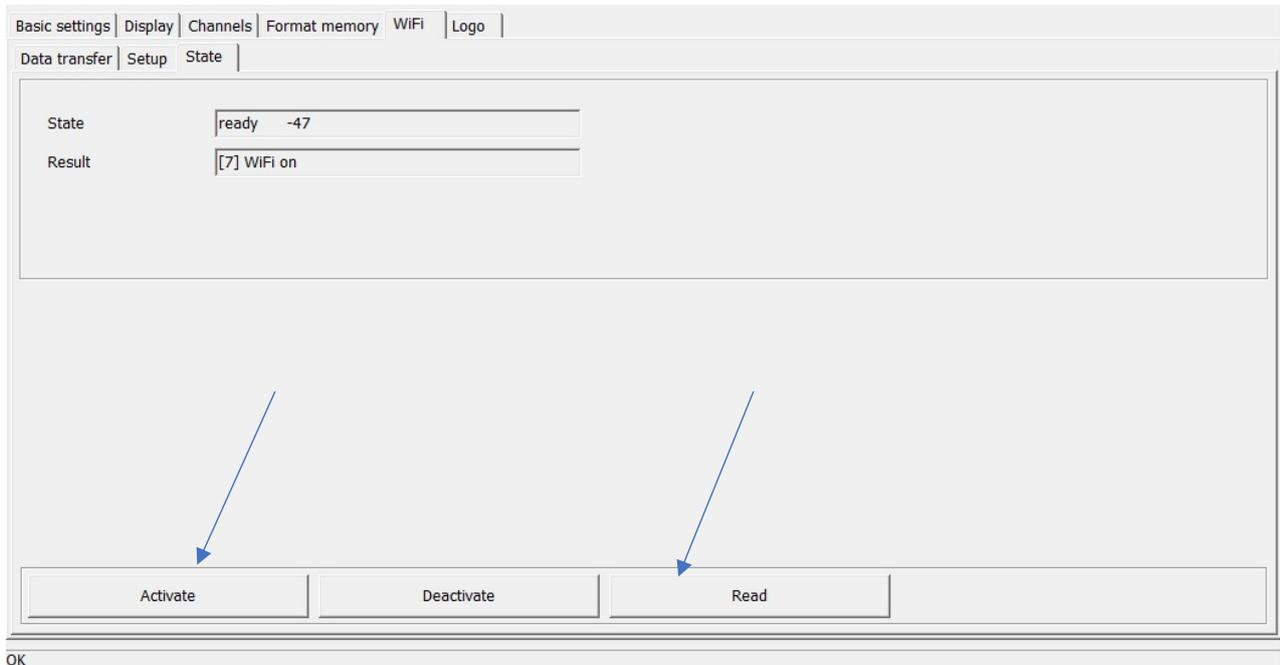
It is recommended to activate and deactivate the logger's WiFi module at the MSR145W2D itself for the period of use:
