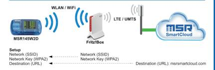
In this option an additional WiFi network and internet access using a mobile phone connection are provided — e.g. through a Fritx!Box. A suitable Fritz!Box as well as a SIM card that can be used in many countries is available from MSR Electronics GmbH upon request. The configuration instruction for the Fritz!Box is available in the support area on www.msr.ch.
