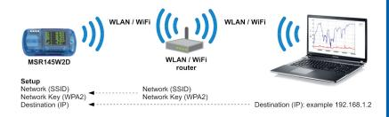
For this option you do not require any additional hardware, as it uses the existing network infrastructure. There is no internet access needed, as the measuring data is sent to a local application.
