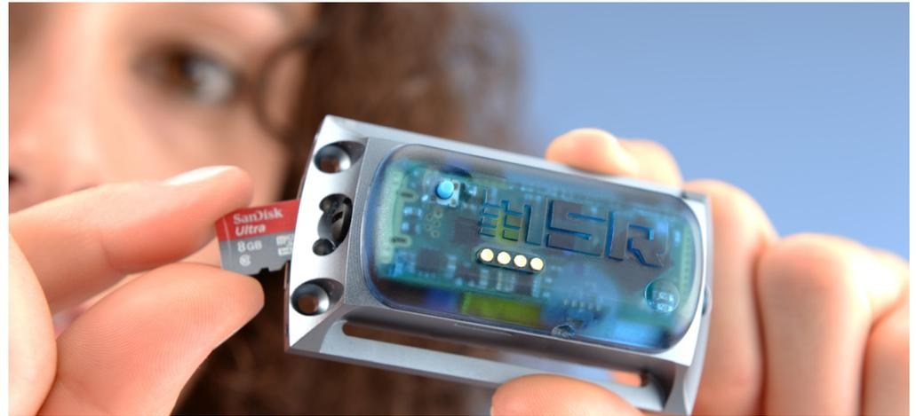
**THE bestseller for transportation monitoring, fault diagnoses and load tests!** The robust MSR 165 data logger is capable of taking 1600 acceleration (shock, vibrations) measurements per second in all three axes for up to five years.
