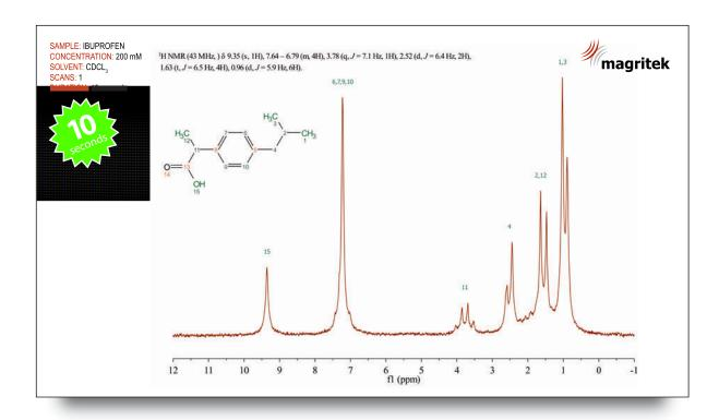
Shown here is a high resolution spectrum of 200 mM ibuprofen dissolved in d-chloroform. It was acquired in a single scan taking just 10 seconds. The lines corresponding to the different protons in the molecule have been completely assigned and the numbers are indicated in the molecule shown in the inset. The methyl peaks at 1 ppm are split by their coupling to the single proton at position 2.
