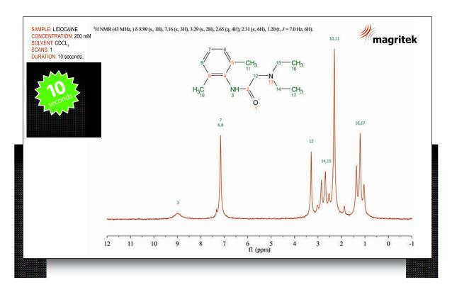
Shown here is an example spectrum of a 200 mM lidocaine sample dissolved in d-chloroform and measured in just 10 seconds. All the spectral features can be observed and resolved. The methyl groups at positions 16 and 17 are resolved completely from the methyl groups at 10 and 11.
