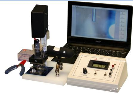
**APPNANO** STM Tip Etcher is a compact, easy to use system for etching custom STM tips with a user controlled timed etch. The etcher features an automatic tip etch stop, an automatic dip and retract, and a live tip etch view. The machine uses pulse etching technology for highly controlled and reproducible tip radius of curvature and aspect ratio. The pulse width is variable for creating custom tip shapes. An optional electroplating mode is capable of nanometer scale metal deposition.
