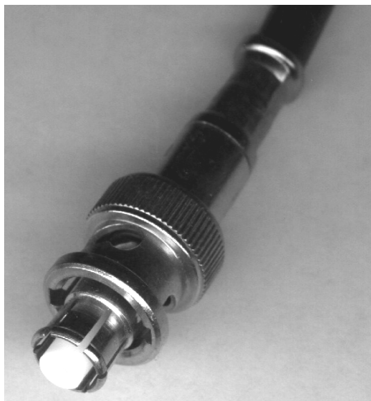
Figure 9. Missing Ground in the SHV Connector.
