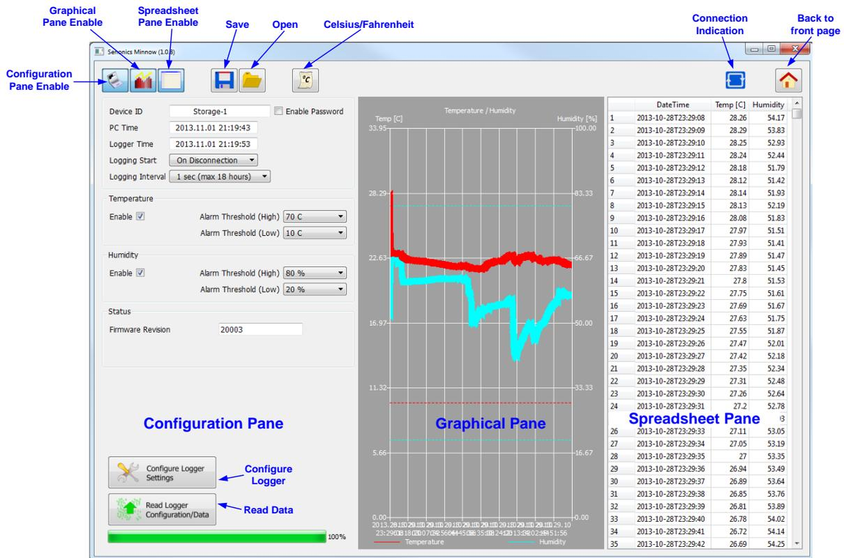
8. Choose a "Logger Start" option, a "Logging Interval" option and any alarms if needed.
