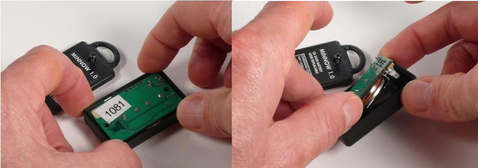
3. Insert the new battery with the + terminal up and then close the back cover. Be careful not to over tighten the screws.
