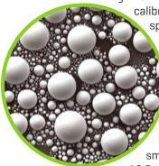
calibration specimen. This is a particularly good resolution test specimen for training new users of SEMs. The ability to image the specimen at low magnification simplifies initial focussing at low accelerating voltages.
