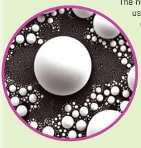
The near perfect round shape of tin spheres is particularly useful for astigmatism correction in a SEM, FESEM or FIB as well as testing image quality, distortion, contrast, brightness and probe size. Tin on Carbon standards are suitable for testing resolution over a wide range of magnifications for most instrument applications. For semiconductor applications where it is not possible to use Gold on Carbon, a Tin on Carbon resolution standard provides an excellent alternative.
