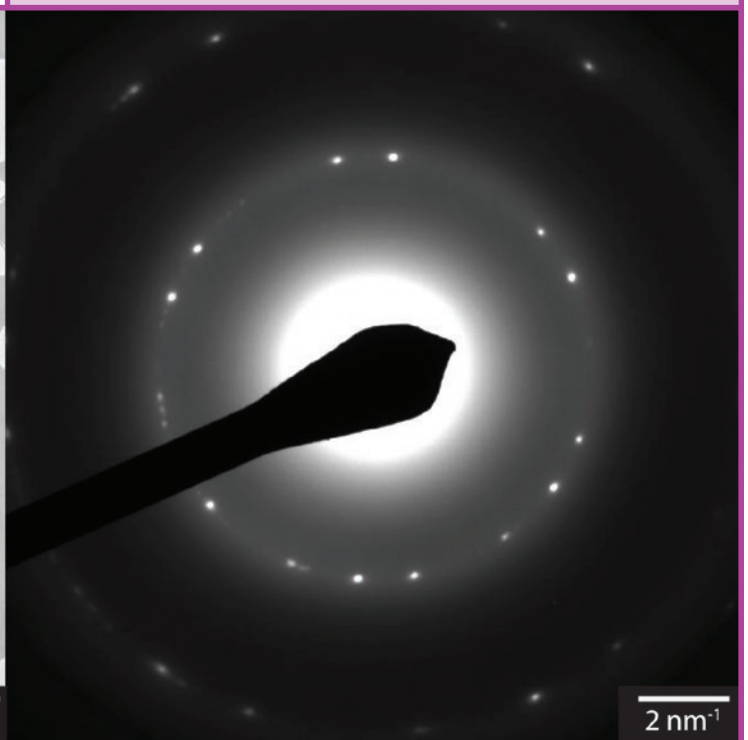
Figure 3. Double layer GO provides a very thin support film for many applications. The diffraction shows a double hexagonal pattern indicating 2-layer GO with complete coverage of this area of the Holey carbon support
